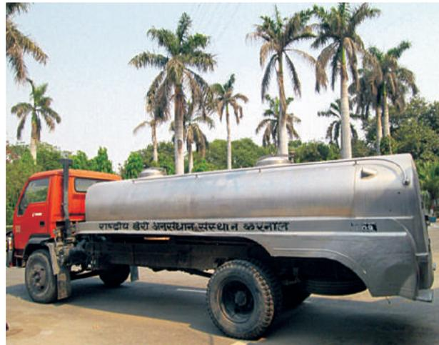
**Fig.3.2. Stainless steel milk tanker**
