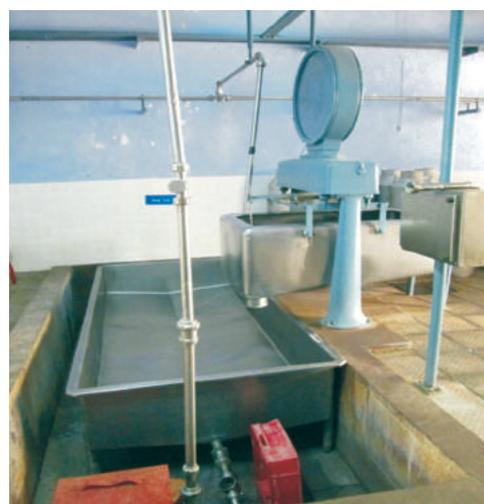
**Fig.3.7. Milk dump tank**
