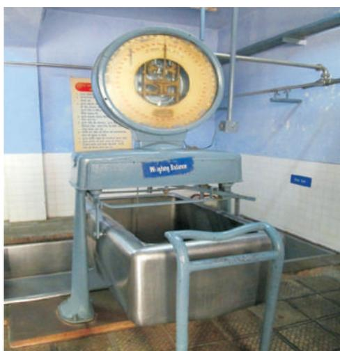
**Fig.3.8. Milk weighing tank**
