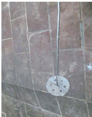
**Fig.3.5. Plunger for mixing of milk**
