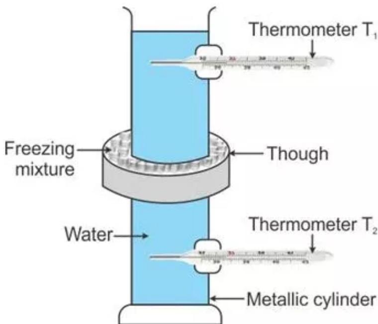
Hope's apparatus consists of a tall metallic cylinder provided with two side openings P and Q, P near the top and Q near the bottom, fitted with thermometers T<sub>1</sub> and T<sub>2</sub> in them. The central part of the cylinder is surrounded with a cylindrical trough containing a freezing mixture of ice and salt. The cylinder is fitted with pure water at room temperature.
