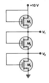
if  $I_D = 0.5$  mA,  $V_1 = 5$  V and  $V_2 = 2$  V then the width to-length ratio required in each transistor are
