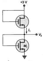
Current  $I_1$  and voltage  $V_2$  are respectively,
