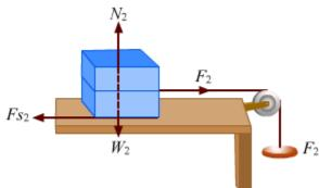
When the block just moves, the applied force is equal to the limiting force of friction.
