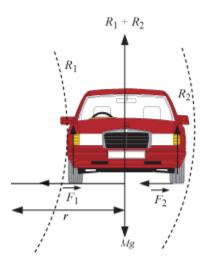
If  $R_1$  and  $R_2$  are the normal reactions of the ground on the two tyres of a car of weight  $M_g$ , going around on a circular turn of radius r, with velocity v, on a level road, then
