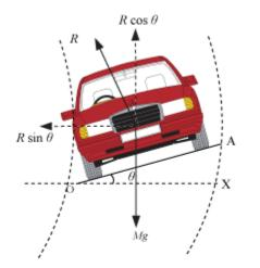
Consider a vehicle of weight Mg, moving round a curved path of radius r, with a speed v, on a road banked through angle  $\theta$ .
