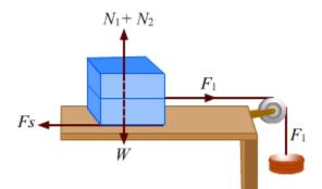
Now, the wooden blocks A and B are placed one after another. In this case, the area of contact increases, but  $W = N_1 + N_2$  remains the same. Weights are added in the pan till the blocks begin to move. Weight  $F_2$  is noted.
