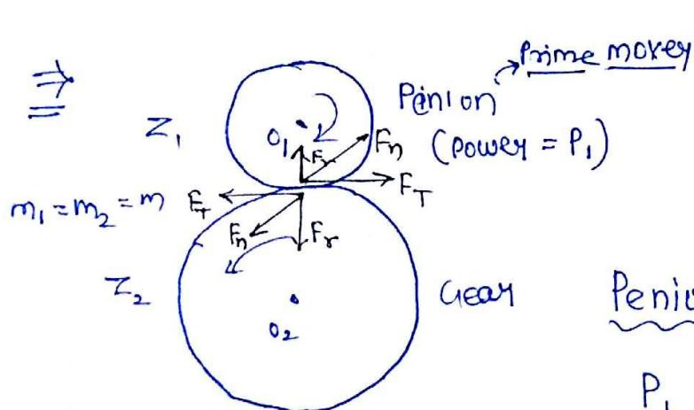
Pinion (small) is generally prime mover because it have low inertial
