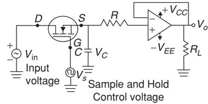
The Analog signal  $V_{in}$  to be sampled is applied to the drain, and sample and hold central voltage ( $V_s$ ) is applied to the gate of E-MOSFET.
