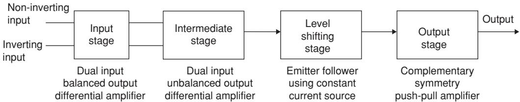
Figure 1 Block diagram of a typical op-amp
