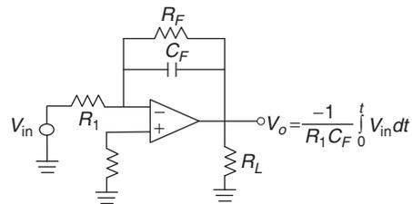
The gain limiting frequency  $f_a = \frac{1}{2\pi R_F C_F}$  and  $R_1 C_F$  values should be selected such that  $f_a < f_b$ .
