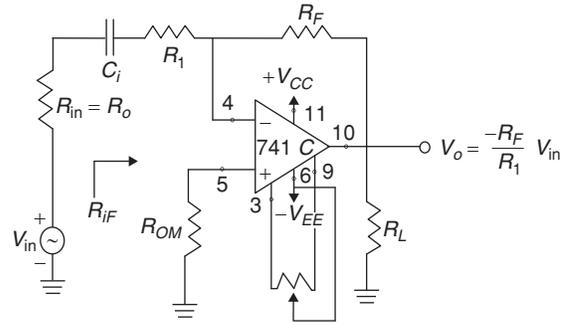
The coupling capacitor not only blocks the DC voltage but also sets the low frequency cutoff limit
