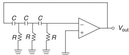
Phase-shift oscillator with three lead circuit in the feedback path, at some frequency the total phase shift of the three
