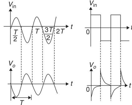
Figure 9 Input-output wave forms
