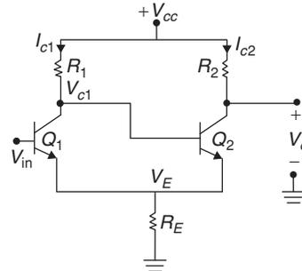
The basic Emitter coupled pair can be converted into a regenerative comparator. The resistances  $R_1$  and  $R_2$  are unequal ( $R_1 > R_2$ ) and hence  $Q_1$  and  $Q_2$  have different currents when saturated. This difference results in the hysteresis as different input voltages are required to saturate and cutoff  $Q_1$  and  $Q_2$ .
