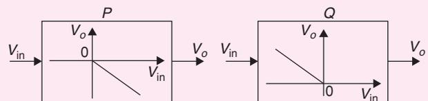
It is desired to make full-wave rectifier using above two half-wave rectifiers. The resultant circuit will be [2008]
