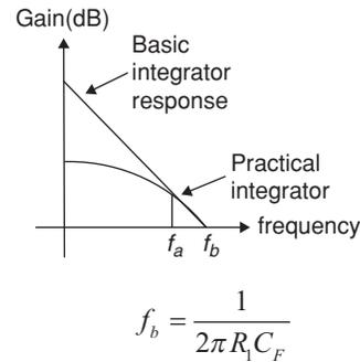
The stability and low frequency roll-off problem can be corrected by the addition of a resistor  $R_F$  as shown in the practical integrator
