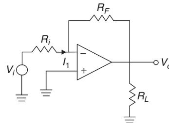
$$I_1 = \frac{V_i}{R_i}, V_o = -I_1 R_f = \frac{-R_f}{R_i} V_i$$
