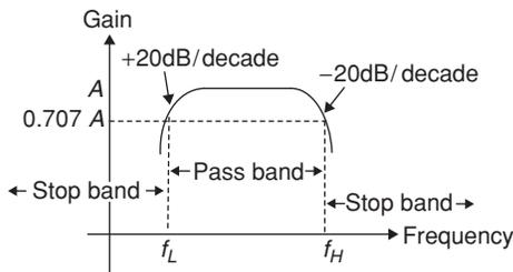
If figure of merit or  $Q$  factor  $Q < 10$ , then the filter is called as wide band pass filter
