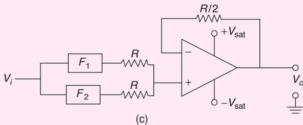
The cut-off frequencies of  $F_1$  and  $F_2$  are  $f_1$  and  $f_2$  respectively. If  $f_1 < f_2$ , the resultant circuit exhibits the characteristics of a
