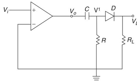
A zero crossing detector converts the sinusoid input ( $V_i$ ) into a square wave, ( $V_o$ )
