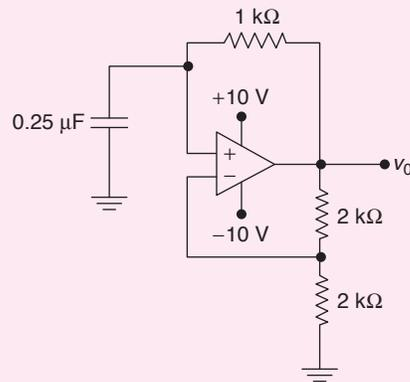
The saturation voltage of the ideal op-amp shown below is  $\pm 10$  V. The output voltage  $v_o$  of the following circuit in the steady-state is
