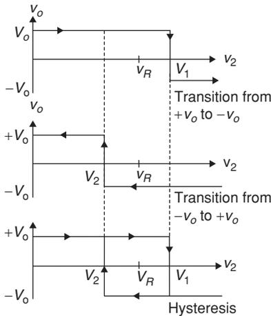
If we decrease  $v_2$ , the output remains at  $-V_o$ , until  $v_2$  equals the voltage at positive terminal, or until  $v_2 = V_2$ . At this stage, regenerative transition takes place and the output returns to  $+V_o$  almost instantly. One of the most important uses made of the Schmitt trigger is to convert a slowly varying input voltage into an output wave from displaying an abrupt, almost discontinuous change.
