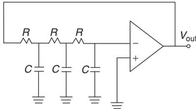
Figure 11 Phase shift oscillator with lag circuits
