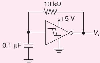
If the lower and upper trigger level voltages are 0.9 V and 1.7 V, the period (in ms), for which output is low, is \_\_\_\_.
