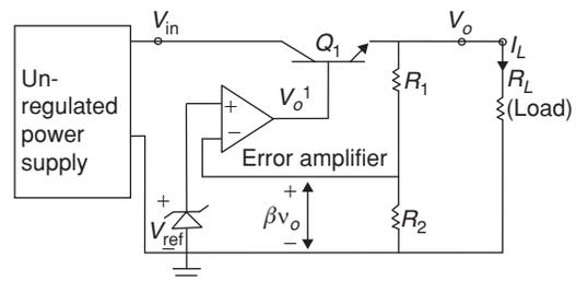
**Figure 13** A regulated power supply
