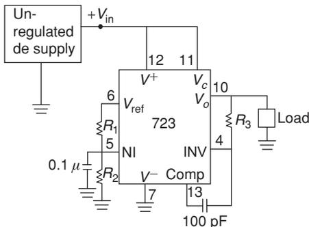
**Example 28:** An op-amp circuit is shown in the figure, the current 'I' is
