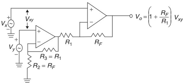
Figure 4 Differential amplifier with two op-amps
