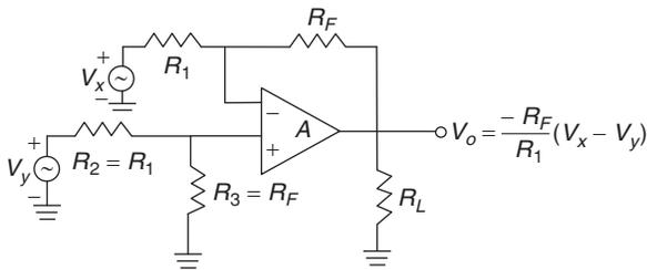
Figure 3 Differential amplifier with one op-amp
