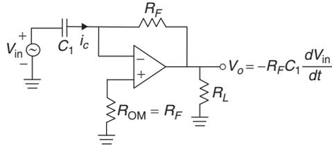
The output  $V_o$  is equal to  $R_F C_1$  times the negative instantaneous rate of change of input voltage  $V_{in}$  with time
