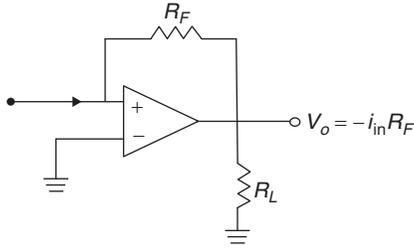
The introduction of negative feedback stabilizes the gain; however, it is also smaller than the open loop gain. On the contrary, positive feedback is necessary in oscillator circuits.
