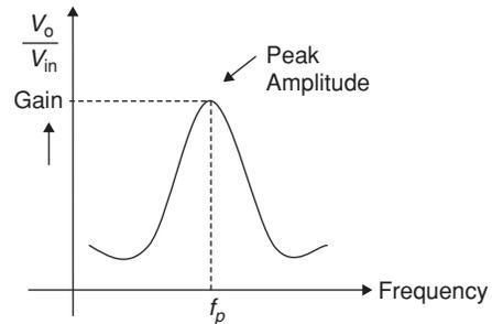
The peaking response, that is the frequency response that peaks at a certain frequency, can be obtained by using a parallel LC network with the op-amp
