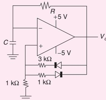
The time duration for +ve part of the cycle is  $\Delta t_1$  and for -ve part is  $\Delta t_2$ . The value of  $e^{\frac{\Delta t_1 - \Delta t_2}{RC}}$  will be \_\_\_\_\_.
