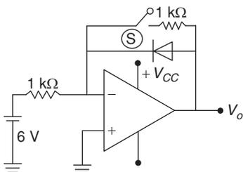
What is the output  $V_o$  when switch 'S' is open
