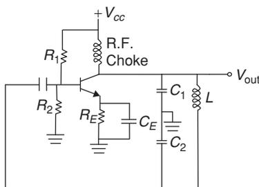
CE connection, Colpitts oscillator resonant frequency
