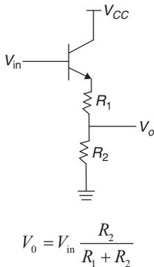
Resistor  $R_2$  not only level-shifts DC by an amount  $\frac{R_2}{R_1 + R_2}$  but also attenuates the AC signal. Remedy is to replace  $R_2$  with current mirror circuit.
