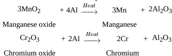
Similarly, chromium is obtained by heating chromium oxide with aluminium powder.
