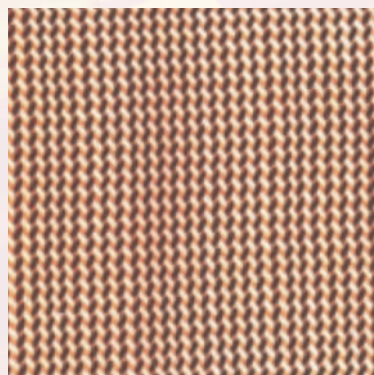
Herring bone woven fabric- a derivatives of twill woven structure Image 26
