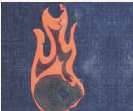
Denim usually having 3/1 twill woven with warp dyed in indigo colour and the weft is off white, now available in various shades of colour. Above the denim is printed with rubber printing technique Image 34
