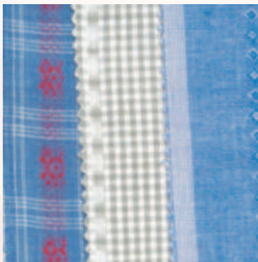
Dobby fabrics with Small buties made on it Image 63
