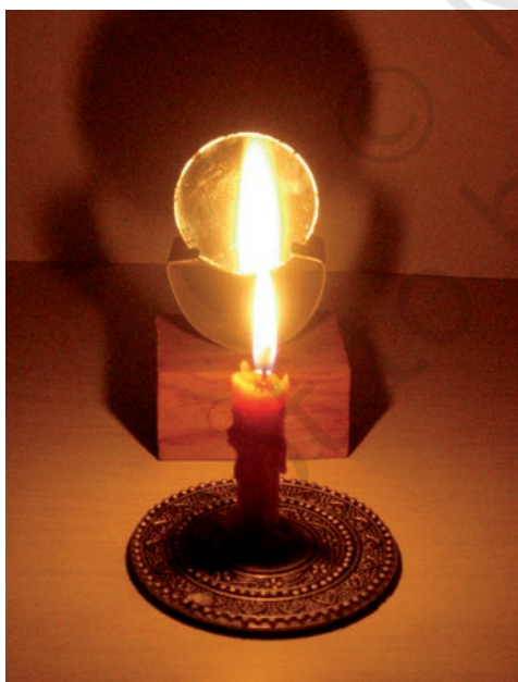
Fig. 15.16 Virtual image formed by a concave mirror
