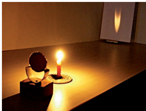
Fig. 15.15 Real images formed by a concave mirror
