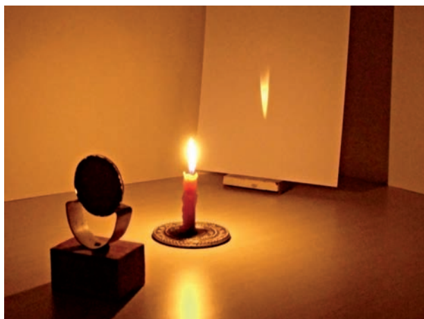
Fig. 15.15 Real images formed by a concave mirror
