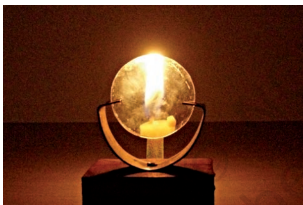
Fig. 15.26 Virtual image formed by the convex lens
