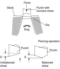
**Example 3:** Calculate the die and punch sizes for blanking a circular disc of 22 mm diameter from a C 20 steel sheet with thickness 1.5 mm. Determine also the punching force (Shear strength for C 20 steel = 294 MPa).
