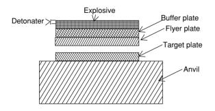
When the explosive is detonated, the flyer plate moves to the target plate under great velocity and bonding occurs with the target plate or base plate. This method is used for metal cladding of heat exchanger tube plates etc. Dissimilar metals can be welded using this method. For example aluminium or copper to stainless steel.
