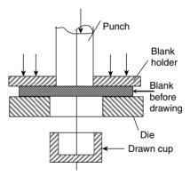
In a single drawing operation the diameter of the blank can be reduced 1.8 to 2 times less than that of the initial blank. If a further reduction is required the blank is to be redrawn.
