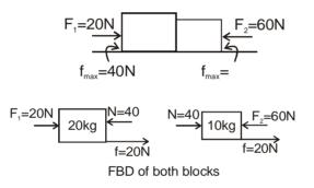
Hence magnitude of friction force on both blocks is 20 N and is directed to right for both blocks. Normal reaction exerted by 20 kg block on 10 kg block has magnitude 40 N and is directed towards right. Net force on system of both blocks is zero.
