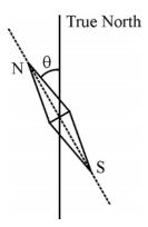
Which element of earth's magnetic field is represented by  $\theta$  in the figure? (1)
