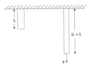
$Longitudinal strain = \frac{l}{T} \ and \ tensile \ stress = \frac{F}{A}$
