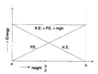
Graphs depicting variations of (i) gravitational potential energy (P.E) (ii) K.E and (iii) the total sum of potential and Kinetic energies for a freely falling body are shown in the diagram.
