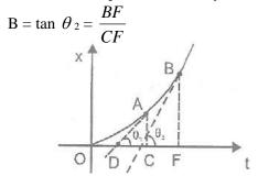
Since  $\theta_2 > \theta_1$ , so slope at B is greater than the slope at A. Hence speed of body at point B is greater than the speed of the body at point A.
