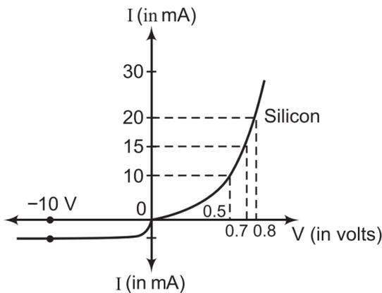
The V-I characteristic of a diode is shown in the figure. The ratio of the resistance of the diode at  $I = 15 \text{ mA}$  to the resistance at  $V = -10 \text{ V}$  is: (CBSE SQP 2023-24)
