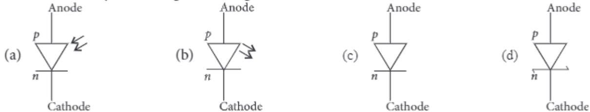
(iii) An LED is constructed from a  $p-n$  junction based on a certain Ga-As-P semiconducting material whose energy gap is 1.9 eV. Identify the colour of the emitted light.
