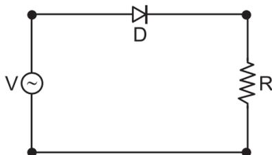
**Q4. What will be the fundamental ripple frequency in a half wave rectifier circuit operating from 50 Hz mains frequency?**
