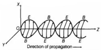
A plane electromagnetic wave travelling along z-axis
