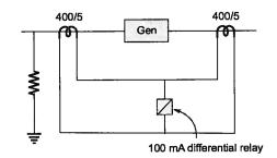
(b) The scheme shown below is used for protection of the generator winding by an ordinary differential relay, having a minimum pick up current of 100 mA. The C.T.s on the grounded neutral and the live ends have actual ratios of 79 and 81 respectively though their nominal ratios are same.
