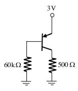
For an emitter base voltage  $V_{EB} = 600 \text{mV}$ , the emitter collector voltage  $V_{EC}$  (in Volts) is \_\_\_\_\_.
