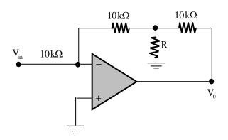
If the gain  $(V_0/V_{in})$  is -12, the value of R (in  $k\Omega$ ) is \_\_\_\_\_\_.
