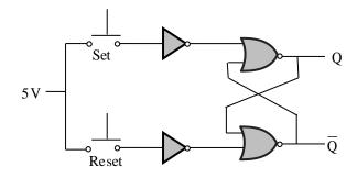
The set and reset pulse inputs are provided using the push-button switches. It is observed that the circuit fails to work as desired. The SR latch can be made functional by changing
