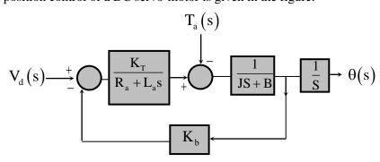
The values of the parameters are  $K_T$ = 1 N-m A,  $R_a$ = 1  $\Omega$ ,  $L_a$ = 0.1H. J= 5 kg-m², B= 1 N-m (rad/sec) and  $K_b$ = 1 V/(rad/sec). The steady-state position response (in radians) due to unit impulse disturbance torque  $T_d$ is \_\_\_\_\_\_.
