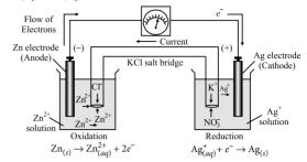
(i) The zinc electrode is negatively charged (anode) as it pushes the electrons into the external circuit.
