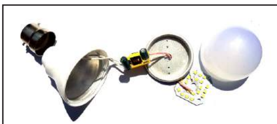
Figure Showing a Completed LED Bulb Circuit
