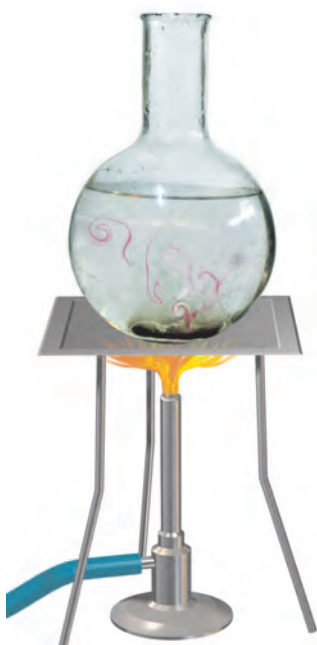
Fig. 4.9 Convection of heat in water
