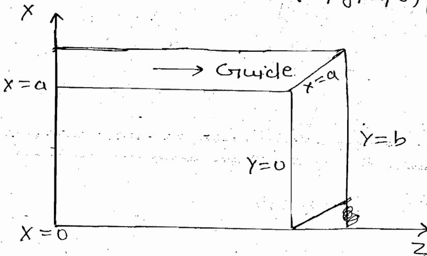
→ It is a single conductor hollow structure used to confine EM wave in 2 dimension using 4 walls
