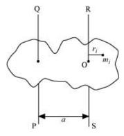
Suppose a rigid body is made up of n particles, having masses  $m_1, m_2, m_3, \ldots, m_n$ , at perpendicular distances  $r_1, r_2, r_3, \ldots, r_n$  respectively from the centre of mass O of the rigid body.
