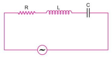
The voltage V = V0 sin  $\omega$ t is applied across the series LCR circuit. However due to impedance of the circuit, either current lags or leads the voltage by phase opposite so the current in the circuit is given by
