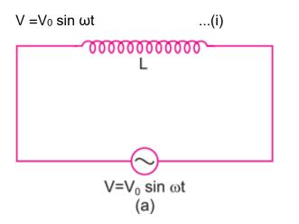
If i is the instantaneous current in the circuit and  $\frac{di}{dt}$  the rate of change of current in the circuit at that instant, then instantaneous induced emf
