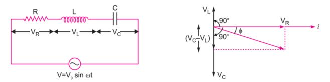
Suppose the voltage across resistance R is V<sub>R</sub> voltage across inductance L is V<sub>L</sub> and voltage across capacitance C is VC. The voltage VR and current i are in the same phase, the voltage V<sub>L</sub> will lead the current by angle 90° while the voltage VC will lag behind the current by angle 90° (fig. b). Clearly VC and VL are in opposite directions, therefore their resultant potential difference = V<sub>C</sub> - V<sub>L</sub> (if V<sub>C</sub> > V<sub>L</sub>)
