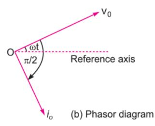
**Phasor diagram:** The phasor diagram of circuit containing pure inductance is shown in Fig. (b).
