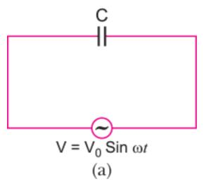
**Circuit Containing Pure Capacitance:** Consider a capacitor of capacitance C; connected to an alternating voltage source as shown.
