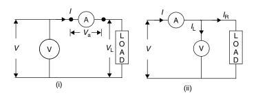
• The power taken by a load from a DC supply is given by the product of readings of an ammeter and voltmeter when connected in a circuit.
