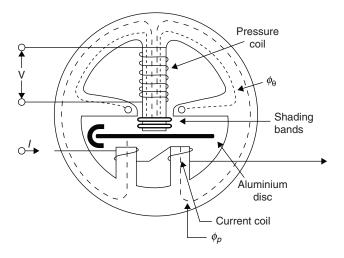
Induction type single-phase energy meter is extensively used to measure energy supplied to a single-phase circuit.
