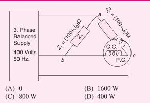
5. A wattmeter is connected as shown in the figure. The wattmeter reads [2010]
