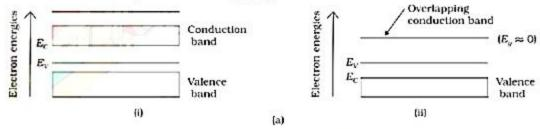
(ii) The valence band is completely filled and the conduction band is empty but the two overlap each other [Fig. a(ii)].
