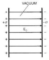
Consider a parallel plate capacitor having vacuum between the plates. Suppose that the capacitor is charged with a battery so that electric field of strength  $E_0$  is set up between the plates as shown in Fig. If  $\sigma$  and  $-\sigma$  are surface charge densities of the two plates of the capacitor, then the electric field between two plates is given by
