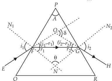
Let  $PQR$  be the principal section of the prism. The refracting angle of the prism is  $A$ .
