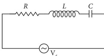
An alternating potential of 100 volts and 50 hertz is applied across a series circuit having an inductance of 5 henry, a resistance of 100 ohm and a variable capacitance.
