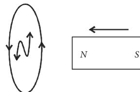
When the N pole of a magnet is moved towards a coil, the induced current in the coil flows in anticlockwise direction on the side of magnet, so as to acquire north polarity and oppose the motion of the magnet towards the coil, by applying repulsive force on it.
