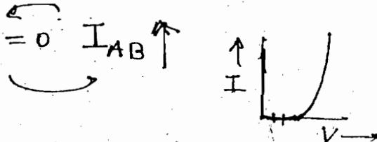
eg:- (i) diode current after cutting voltage
