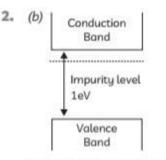
**Explanation:** In *n*-type semiconductor impurity energy level lies just below the conduction band.
