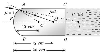
i.e. the curved surface will form virtual image I at distance of 30 cm from P. Since the image is virtual there will be no refraction at the plane surface CD (as the rays are not actually passing through the boundary), the distance of final image I from P will remain 30 cm.
