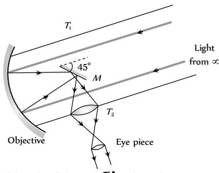
If  $f_o$  is focal length of the concave spherical mirror used as objective and  $f_e$  the focal length of the eye-piece, the magnifying power of the reflecting telescope is given by  $m = \frac{f_o}{f_e}$
