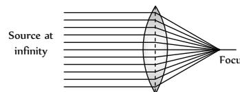
34. (a) The focal length of a lens is given by  $\frac{1}{f} = (\mu - 1) \left( \frac{1}{R_1} - \frac{1}{R_2} \right)$
