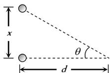
47. (c)  $\frac{1.22 \lambda}{a} = \frac{x}{d} \Rightarrow d = \frac{x \times a}{1.22 \lambda} = \frac{1 \times 10^{-3} \times 3 \times 10^{-3}}{1.22 \times 500 \times 10^{-9}} = 5 \text{ m}$
