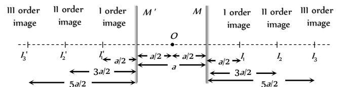
From above figure it can be proved that separation between  $n$ th order image formed in the two mirrors =  $2na$
