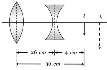
Hence for concave lens  $u = +4 \text{ cm}$ ,  $f = 20 \text{ cm}$ . So by lens formula  $\frac{1}{-20} = \frac{1}{v} - \frac{1}{4} \Rightarrow v = 5 \text{ cm}$  i.e. distance of final image ( $I_2$ ) from concave lens  $v = 5 \text{ cm}$  by using
