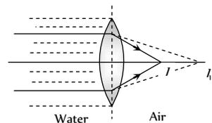
$$1 - \frac{3}{2} = \frac{3}{-R} + \frac{1}{v_2} \Rightarrow v_2 = \left(\frac{3}{2}\right)R$$
