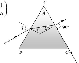
70. (c) In both A and B, the refracted ray is parallel to the base of prism.
