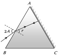
75. (a) From figure it is clear that TIR takes place at surface AC and BC
