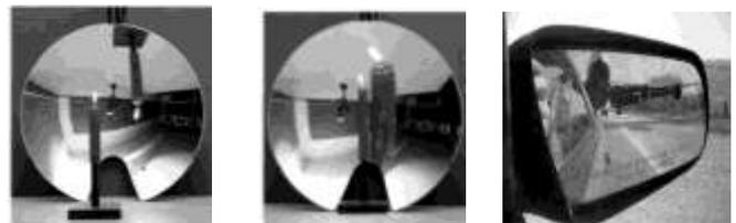
**Concave mirror** : Image formed by concave mirror may be real or virtual, may be inverted or erect, may be smaller, larger or equal in size of object.
