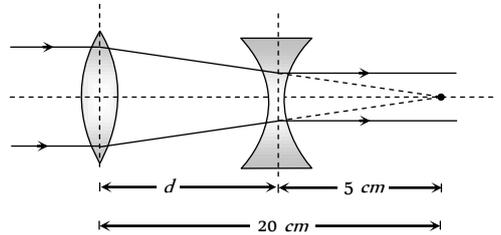
19. (c) According to lens formula  $\frac{1}{f} = (\mu - 1) \left[ \frac{1}{R_1} - \frac{1}{R_2} \right]$
