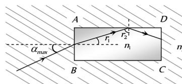
$$\frac{n_1}{n_2} = \frac{\sin \alpha_{\max}}{\sin r_1} \Rightarrow \alpha_{\max} = \sin^{-1} \left[ \frac{n_1}{n_2} \sin r_1 \right] \quad \dots(i)$$
