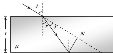
The Lateral shift of the ray is the perpendicular distance between the incident and the emergent ray, and is **Fig. 29.25**
