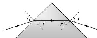
37. (b) The velocity of light in a material medium depends upon its colour (wavelength). If a ray of white light is incident on a prism, then on emerging, the different colours are deviated through different angles.
