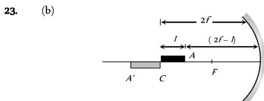
End  $A$  of the rod acts as an object for mirror and  $A'$  will be its image so  $u = 2f - l = 20 - 5 = 15 \text{ cm}$
