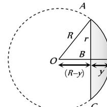
If  $r$  is the radius and  $y$  is the thickness of lens (at the centre), the radius of curvature  $R$  of its curved surface in accordance with the figure is given by
