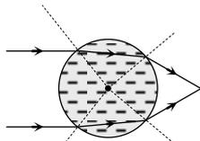
8. (a) When light ray goes from denser to rarer medium (i.e. more  $\mu$  to less  $\mu$ ) it deviates away from the normal while if light ray goes from rarer to denser medium (i.e. less  $\mu$  more  $\mu$ ) it bend towards the normal.
