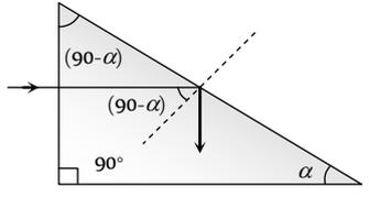
$(90^\circ - \alpha) = C =$  minimum value of angle of incidence at hypotenuse for total internal reflection
