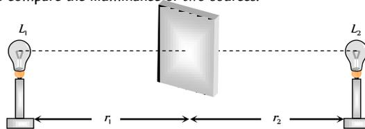
Two sources of luminous intensity  $L_1$ , and  $L_2$  are placed at distances  $r_1$  and  $r_2$  from the screen so that their flux are perpendicular to the screen. The distance  $r_1$  and  $r_2$  are adjusted till  $I_1 = I_2$ . So
