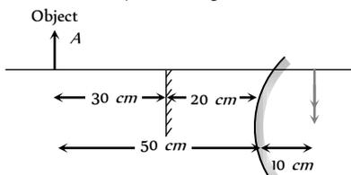
According to property of plane mirror it will form image at a distance of  $30 \text{ cm}$  behind it. Hence for convex mirror  $u = -50 \text{ cm}$ ,  $v = +10 \text{ cm}$
