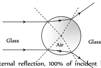
25. (a) In total internal reflection, 100% of incident light is reflected back into the same medium, and there is no loss of intensity, while in reflection from mirrors and refraction from lenses, there is always some loss of intensity. Therefore images formed by total internal reflection are much brighter than those formed by mirrors or lenses.
