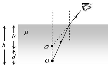
(i)  $\mu = \frac{\text{Real depth}}{\text{Apparent depth}} = \frac{h}{h'}$  **Fig. 29.21**
