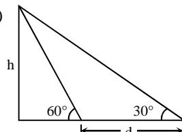
$$d = h \cot 30^\circ - h \cot 60^\circ \text{ and time} = 3 \text{ min.}$$
