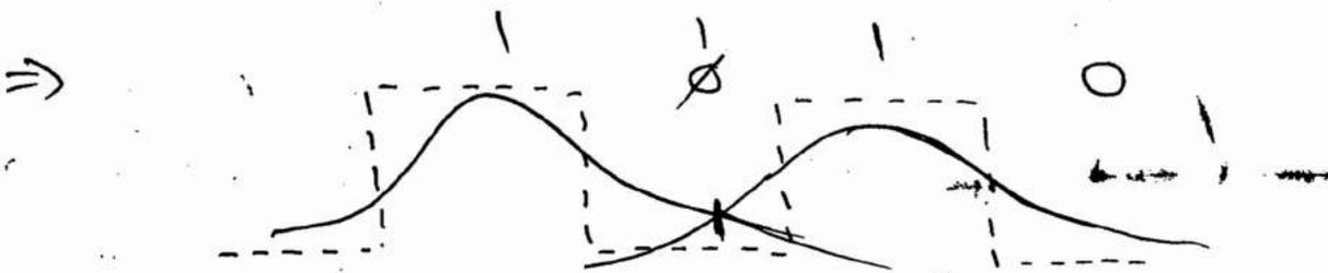
⇒ Due to ~~this~~ pulse dispersion, overlapping occurs and this phenomenon is called as the Inter Symbol Interference.
