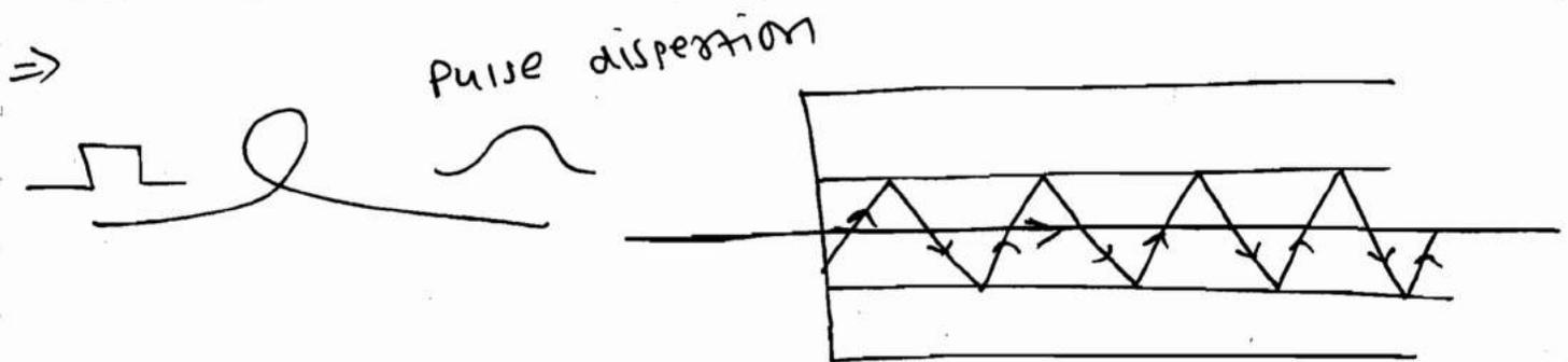
⇒ Assume that the binary data 101011 is transmitted through a fiber optic cable. Due to pulse dispersion the signal at the o/p will as shown in fig.
