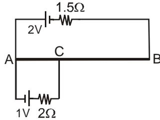
6. Potential gradient of the part CB of the wire is :
