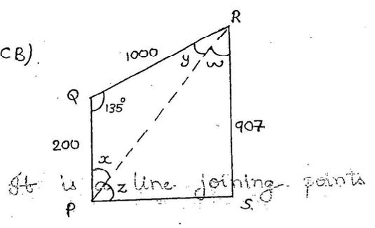
$$\begin{aligned} \angle PQR &= (BB)_{PQ} - (FB)_{QR} \\ &= (180+0) - 45 = 135^\circ \end{aligned}$$
