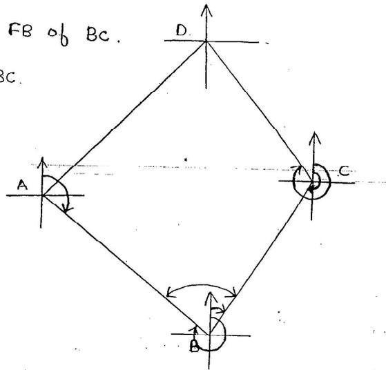
\* Calculation of Bearings from given interior angles.
