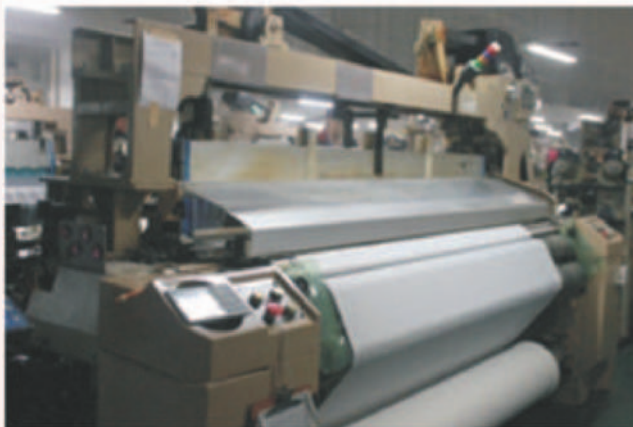
Fig 3.6: Waterjet Loom - Observe the lustre on the fabric, it is because the fabric is wet due to water.
