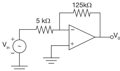
Consider the op-amp input offset voltage  $V_{io} = 1.5$  mV.
