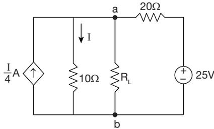
The Norton's equivalent model of the circuit across  $R_L$  is \_\_\_\_\_.
