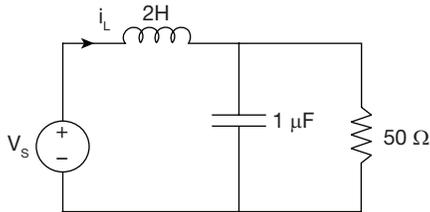
If  $V_s = 5 + 10u(t)$ , then the value of  $\frac{di_L}{dt}$  at  $t = 0^+$  is \_\_\_\_\_ A/S.
