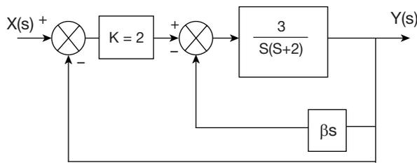
if the damping ratio of the system is equal to 0.5, then the value of  $\beta$  is .....
