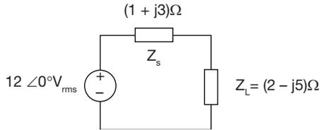
The reactive power consumed by the load  $Z_L$  is \_\_\_\_\_.
