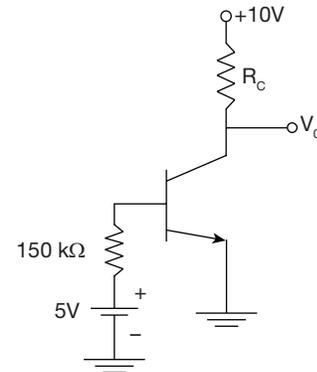
The value of  $R_C$  for which the transistor remains in saturation region is \_\_\_\_\_.
