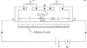
We move the jockey, on the wire of the meter bridge, till we find a point at which the deflection in G, is zero, we can have(value of R is known to us)
