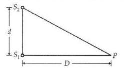
The path difference is maximum when the detector lies at point S<sub>1</sub>.
