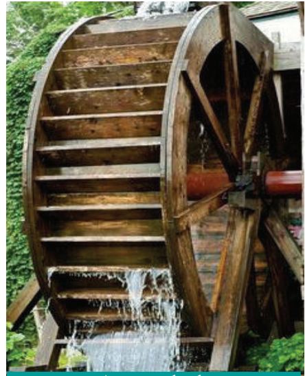
A water wheel used for irrigation
