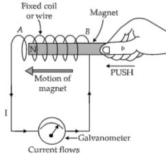
(i) A student connects a coil of wire with a sensitive galvanometer as shown in figure. He will observe the deflection in the galvanometer if bar magnet is
