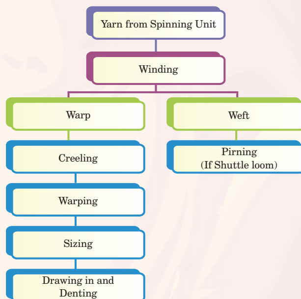
Fig 4.1: Flow chart for Yarn Preparatory Process
