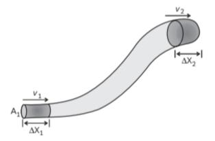
Bernoulli's theorem, in fluid dynamics, relation among the pressure, velocity and elevation in a moving fluid (liquid or gas), the compressibility and viscosity of which are negligible and the flow of which is steady, or laminar. Bernoulli's principle is applicable to those non-viscous liquids which have laminar or streamlined flow. It means that a liquid in which its particles exert no force on each other i.e. the speed of all particles of the liquid is the same.
