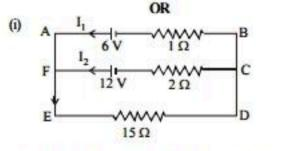
(ii) Applying Kirchhoff's 1st law at pointF, I<sub>1</sub> + I<sub>2</sub> = I<sub>3</sub> .....(1) For the loop ABCFA, applying Kirchhoff's 2nd law, 12 - 6 = -1I<sub>1</sub> + 2I<sub>2</sub> ⇒ 6 = 2I<sub>2</sub> - I<sub>1</sub> ....(2)
