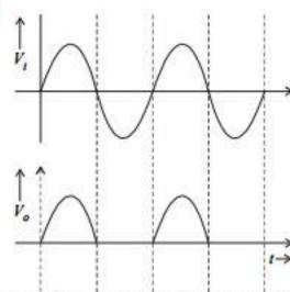
We can see from graph, of input and output of Half Wave Ractifier
