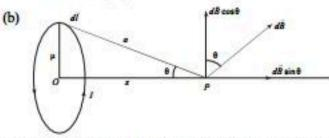
From Biot-savart law, the magnetic field at point P(x, 0, 0)due to current element dl,
