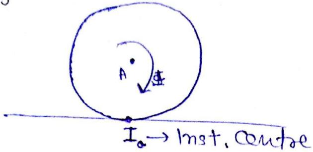
$$\begin{aligned} (\text{K.E.})_{\text{Rolling}} &= (\text{K.E.})_{\text{trans.}} + (\text{K.E.})_{\text{rot-a.}} \\ &= \frac{1}{2} m v_A^2 + \frac{1}{2} I_A \omega^2 \end{aligned}$$
