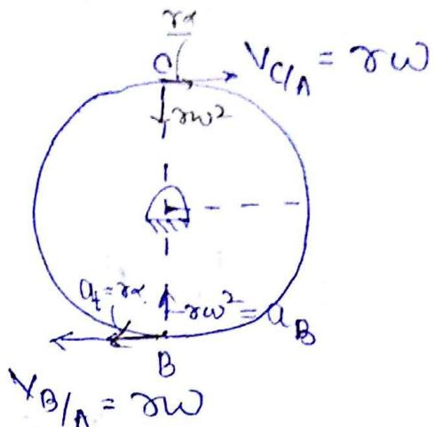
Ques A wheel of radius of 2 m rolls freely as shown in fig if  $V_A = 6 \text{ m/s}$  &  $a_A = 20 \text{ m/s}^2$  then what are the Velocity and acc<sup>n</sup> at point B and C
