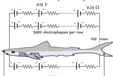
The water surrounding the eel completes a circuit between the head and its tail. If the water surrounding it has a resistance of 500  $\Omega$ , the current an eel can produce in water is about
