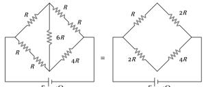
Clearly, the network of resistances is a balanced Wheatstone bridge. So  $R_{AB}$  is given by
