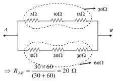
106. (a) The given circuit is a balanced Wheatstone bridge type, hence it can be simplified as follows
