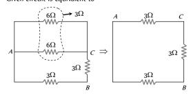
So the equivalent resistance between points A and B is equal to  $R = \frac{6 \times 3}{6 + 3} = 2\Omega$
