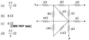
**27.** The effective resistance between points *P* and *Q* of the electrical circuit shown in the figure is
