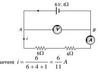
P.D. between A and B,  $V = \frac{6}{11} \times 10 = \frac{60}{11} V$ .
