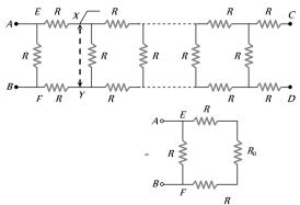
The resistance across  $EF = R_{EF} = (R_0 + 2R)$
