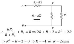
**31.** (b) Cut the series from XY and let the resistance towards right of XY be  $R_0$  whose value should be such that when connected across AB does not change the entire resistance. The combination is reduced to as shown below.
