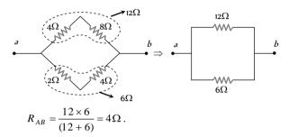
**94.** (d) The given circuit is a balanced wheatstone bridge circuit. Hence potential difference between *A* and *B* is zero.
