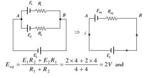
$R_{eq} = \frac{4}{2} = 2\Omega$ . Current  $i = \frac{2+2}{2} = 2A$  from A to B
