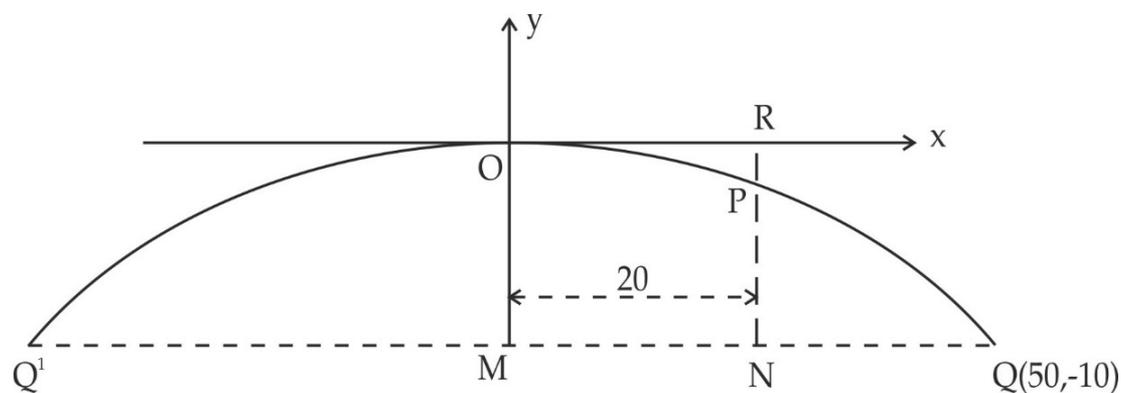
Take the vertex O of the parabola as origin and the axis of the parabola as y-axis. Therefore, the equation of the parabola is  $x^2 = -4ay$ .
