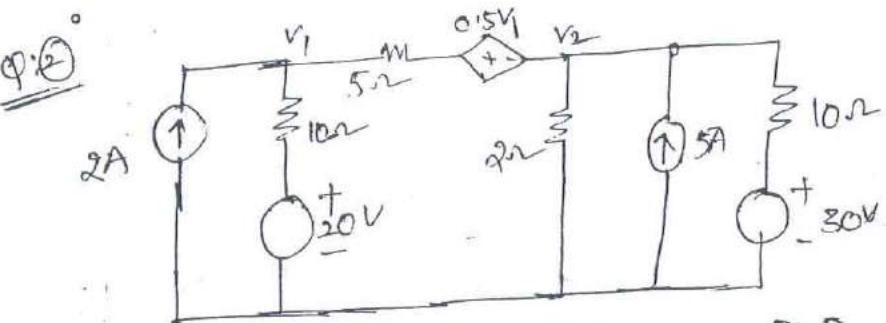
Sol:  $\frac{V_1 - 20}{40} + \frac{V_1 - V_2 - 0.5V_1}{5} = 2 \rightarrow \textcircled{1}$  } from  $\textcircled{1} \& \textcircled{2}$
