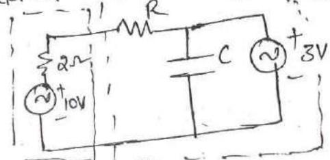
In the figure shown at what value of 'R' power delivered from ckt 'A' to ckt 'B' is max?
