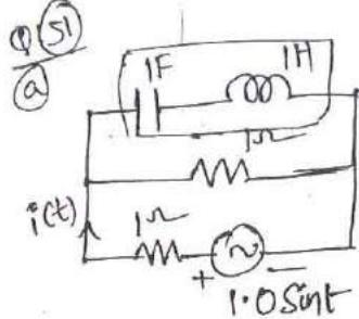
$$\begin{aligned} Z_1 &= j(X_L - X_C) \\ &= j(\omega L - \frac{1}{\omega C}) \\ &= j(1 - 1) \\ &= 0 \end{aligned}$$
