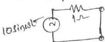
$$\begin{aligned} P &= \frac{(10/\sqrt{2})^2}{(1\Omega)} \\ &= 50W \end{aligned}$$
