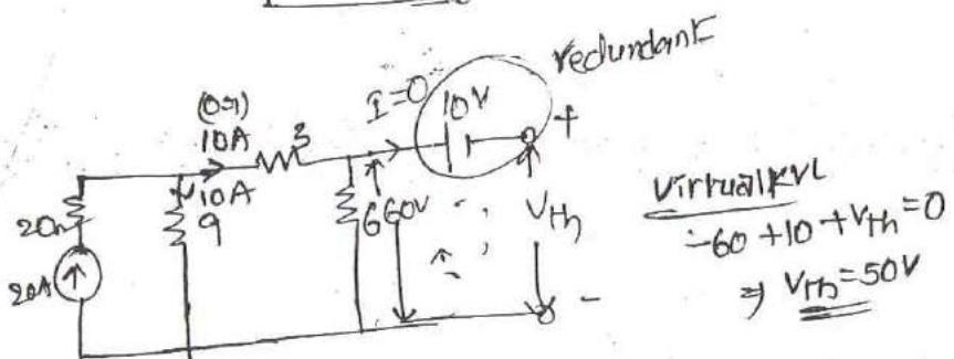
Note:- \* Disconnect the load resistor & find open circuit voltage across the load terminals.
