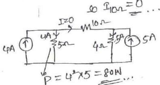
By using source transformation response is obtained in the load resistor, but not in the internal resistor.
