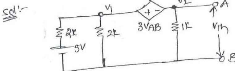
$$\frac{V_1 - 5}{2k} + \frac{V_1}{2k} + \frac{V_2}{1k} = 0 \quad (1)$$
