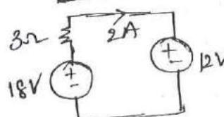
so res is replaced by a voltage source with that res.
