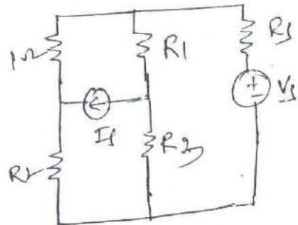
In the circuit shown power dissipation in the  $I_2$  resistor is 576 W, when voltage source is acting alone. If power dissipation in the  $I_2$  resistor is 1 W when current source is acting alone. Find total power dissipation in the  $I_2$  resistor?
