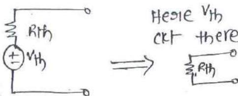
Here  $V_{Th}$  is independent source, but in the given ckt there is no independent source. So  $V_{Th} = 0$ .
