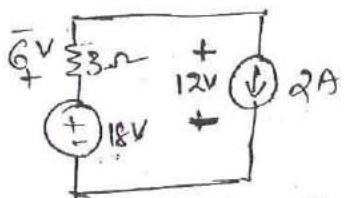
resistance is replaced by eqv current source
