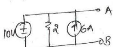
$$V_{AB} = 10V = V_{OC}$$
