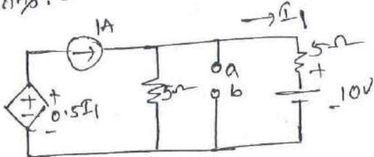
$$I = \frac{V_{Th}}{5} + \frac{V_{Th}-10}{5} \Rightarrow V_{Th} = 7.5 \text{ V}$$
