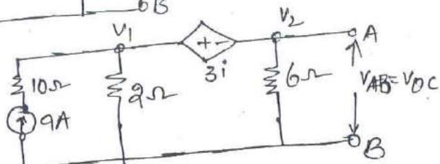
$$\frac{V_1}{2} + \frac{V_2}{6} = 9 \rightarrow ①$$
