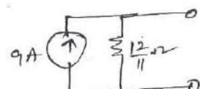
$$\therefore R_{th} = \frac{V_{OC}}{I_{SC}} = \frac{108}{9/10} = \frac{12}{11} \Omega$$
