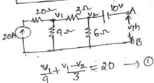
$$\frac{V_1 + V_1 - V_2}{9} = 20 \rightarrow ①$$
