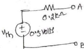
While finding  $R_{th}$  make all independent voltage sources as replaced with their internal res.
