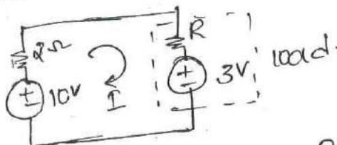
\* for max power transfer  $R_{eq,load} = 2\Omega$
