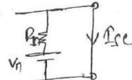
$$I_{SC} = I' = \frac{V_1}{R_1} + \frac{V_2}{R_2} + \dots + \frac{V_n}{R_n}$$
