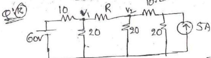
$$\text{so } \underline{V_1 = 40 \text{ when } R = 10\Omega}$$
