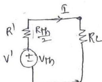
$$I = \frac{V_{th}}{R_{th} + R_L} = \frac{2V_{th}}{R_{th} + 2R_L} \dots$$
