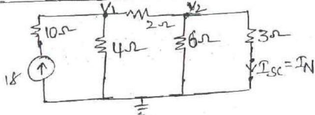
$$\frac{V_1}{4} + \frac{V_1 - V_2}{2} = 18 \rightarrow (1)$$
