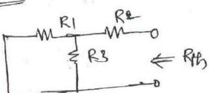
$$\begin{aligned} R_{th} &= (R_1 || R_3) + R_2 \\ &= \frac{R_1 R_3}{R_1 + R_3} + R_2 \end{aligned}$$
