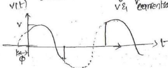
$$\text{Sol: } v_{\text{avg}} = \frac{1}{2\pi} \left[ \int_0^{\pi} v_m \sin(\omega t + \phi) d\omega t + \int_0^{\pi} 0 \right]$$
