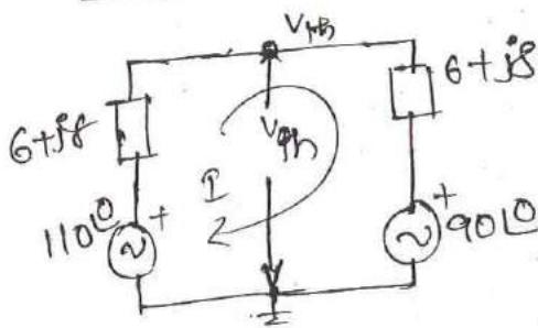
$$\text{Req. } \frac{V_{th} - 110}{6+j8} + \frac{V_{th} - 90}{6+j8} = 0$$
