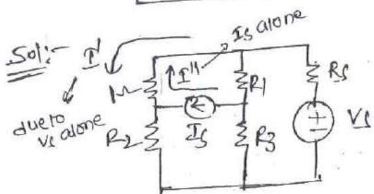
$$\begin{aligned} \text{S.P.T.} &= I^1 + I^{II} \\ V &= \pm V^1 \pm V^{II} \\ P &= \pm P^1 \pm P^{II} \end{aligned}$$
