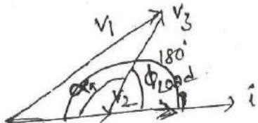
$$V_1 = \sqrt{V_2^2 + V_3^2 + 2V_2V_3 \cos \alpha}$$
