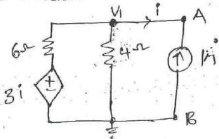
$$R_{Th} = R_{AB} = \frac{V_{AB}}{I_{AB}}$$
