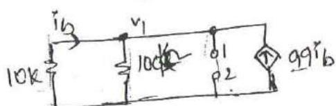
$$R_{th} = \frac{V_{oc}}{I_{sc}} \quad V_{oc} \Rightarrow ?$$
