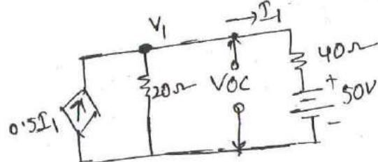
$$\frac{V_1 - 50}{40} + \frac{V_1}{20} = 0.5\Omega_1$$
