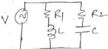
$$\frac{\omega L}{R_1^2 + (\omega L)^2} = \frac{(1/\omega C)}{R_2^2 + (X_{SC})^2}$$
