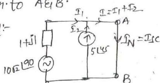
$$I_1 = \frac{10 \angle 190^\circ}{j2 + j1} = 10 \angle 145^\circ$$
