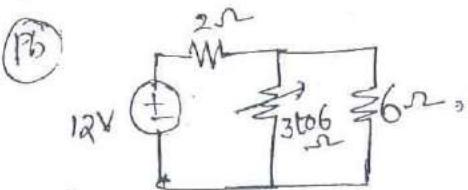
find change in current in the  $\frac{1}{2}\Omega$  &  $6\Omega$  branch when resistance in the variable branch is changed from  $3\Omega$  to  $6\Omega$ .
