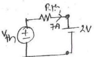
$$\begin{aligned} -v_{th} + 7R_{th} + 2 &= 0 \\ -7R_{th} + v_{th} &= +2 \rightarrow \textcircled{2} \end{aligned}$$
