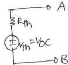
In any linear bidirectional circuit having more number of passive elements, it can be replaced by single equivalent circuit consisting of equivalent voltage source ( $V_{th}$ ) in series with equivalent resistance ( $R_{th}$ ).
