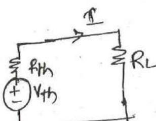
$$P = I^2 R_L = \left( \frac{V_{th}}{R_{th} + R_L} \right)^2 R_L \rightarrow ①$$
