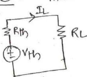
$$I_L = \frac{V_{th}}{R_{th} + R_L} \rightarrow ③$$
