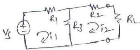
$$V_s = (R_1 + R_3)I_1 - R_3 I_2 \rightarrow (5)$$
