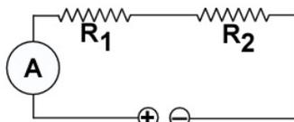
If current  $I$  is drawn from the battery, the current through each resistor will also be  $I$ .
