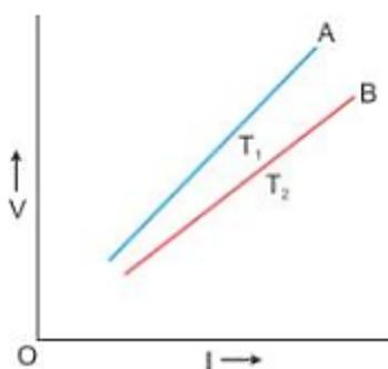
In the above graph,  $T_1 > T_2$ . The straight line A is steeper than the line B, which leads us to conclude that the resistance of conductor is more at high temperature  $T_1$  than at low temperature  $T_2$ . Thus, we can say that resistance of a conductor increases with the increase in temperature.
