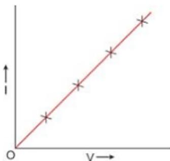
The slope of I-V graph ( $= \frac{\Delta I}{\Delta V}$ ) is equal to the reciprocal of the resistance of the conductor, i.e.
