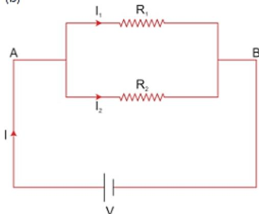
$R_1$  and  $R_2$  are connected in parallel
