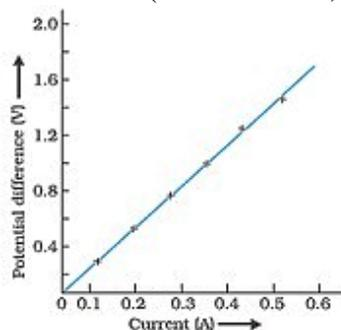
From above graph resistance is determined in the form of slope.
