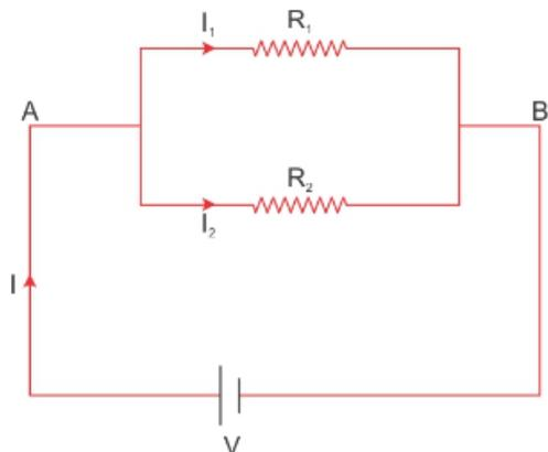
On applying Ohm's law to the two resistors separately, we further
