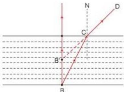
Let any object B is at the bottom of a pond. Consider a light ray BC from the object that moves from water to air. After refraction from the water surface, the ray moves away from the normal N along the path CD. The produce of CD appears from the point B' and a virtual image of the object at B appears at B'.
