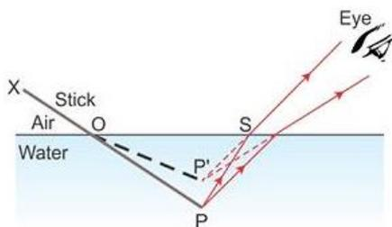
A stick partially immersed in water in a glass container appears bent or raised as shown in figure above. This happens because the rays appear to come from P' (which is the virtual image of the tip P of the stick) due to refraction from denser medium (water) to rarer medium (air) at the surface separating two media.
