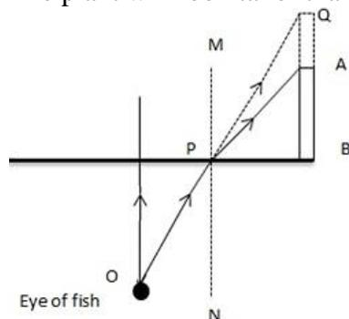
Let the fish is looking from the point O. As the ray OP emerges out from water to air, it will bend away from the normal MN because air is a rarer medium in comparison of water. But if we extend ray OP then it will meet at Q due to which the plant AB will look taller than its actual height.
