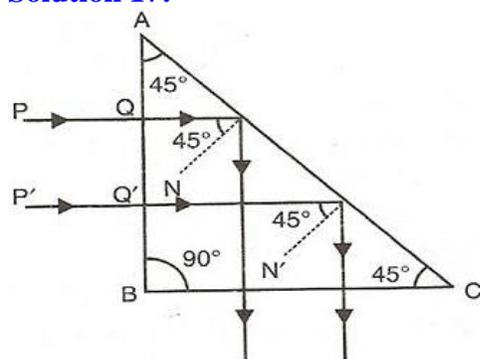
As shown in diagram, a beam of light is incident on face AB of the prism normally so it passes undeviated and strikes the face AC where it makes an angle of  $45^\circ$  with the normal to AC. Because here the incident angle is more than critical angle so rays suffer total internal reflection and reflect at angle of  $45^\circ$ . The beam then strikes face BC, where it is incident normally and so passes undeviated. As a result the incident beam gets deviated through  $90^\circ$ .
