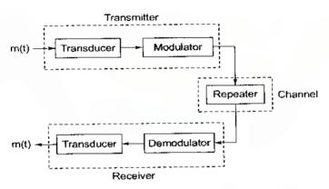
Communication system basically consists transmitter, channel and receiver.
