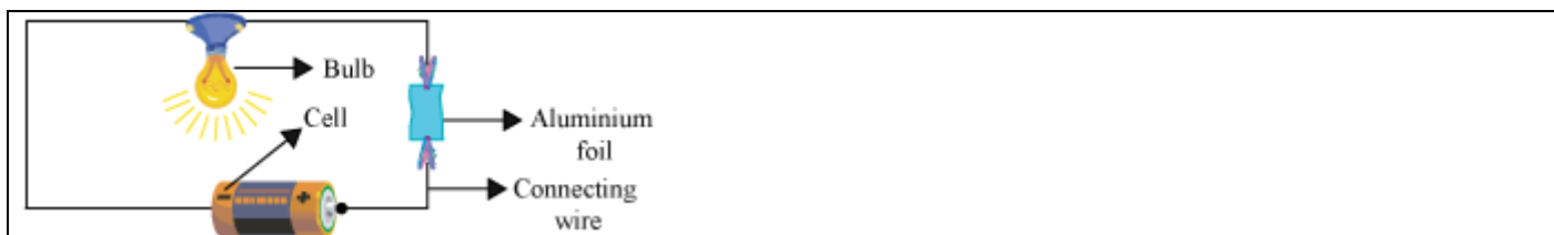
Figure 2: Conduction of electricity in metals
